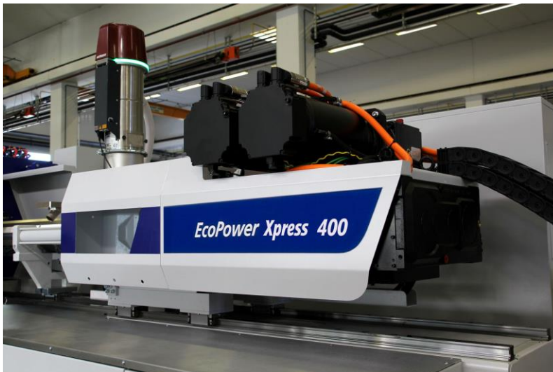
Fig. 2: Highly dynamic injection unit of the new EcoPower Xpress
